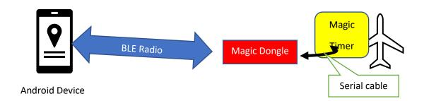
The Dongle is used on the ground to program the timer and is removed before flight. One Dongle will do all your timers. There is a BLE radio in the dongle so it can connect with Super Magic 6 on the Android. The Dongle has a 2.5mm socket and a male to male cable connects the Dongle to the timer.
