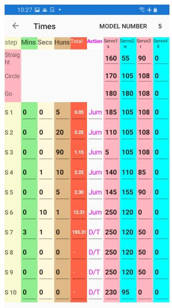
One of the most important and complex changes is on the timer's steps. This screen shows all the steps and the times for the step, servo action and each servo position for that step. This screen has a lot of information.
